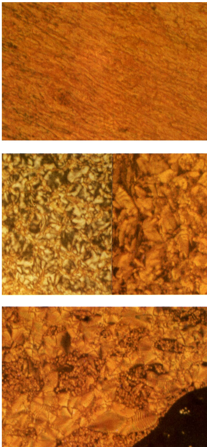
Figure 2. Textures of polymer 9 (crossed polarizers) at (a) 140°C in the cholesteric phase, and (b) at 130°C in the smectic phase; polymer 6 (c) at 134°C in the smectic phase.
